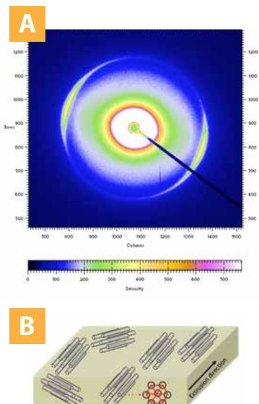
Figure 1 A) 2D SAXS pattern and B) proposed model, for the HCP scattering objects in extruded wheat gluten bioplastic films containing ammonium hydroxide and salicylic acid.
