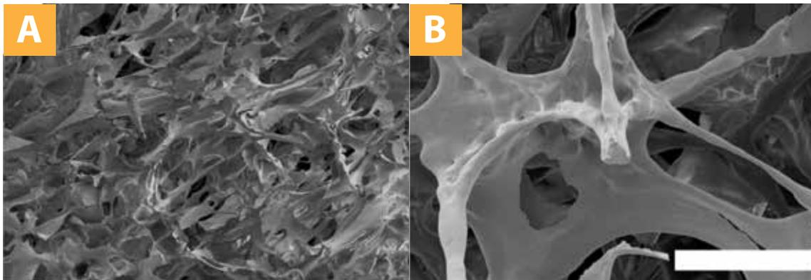
**Figure 2** Freeze-dried WG foams with different protein mixtures observed by Scanning Electron Microscopy (SEM). The gliadin content is higher in **B**. The scale bar in B is 300µm.
