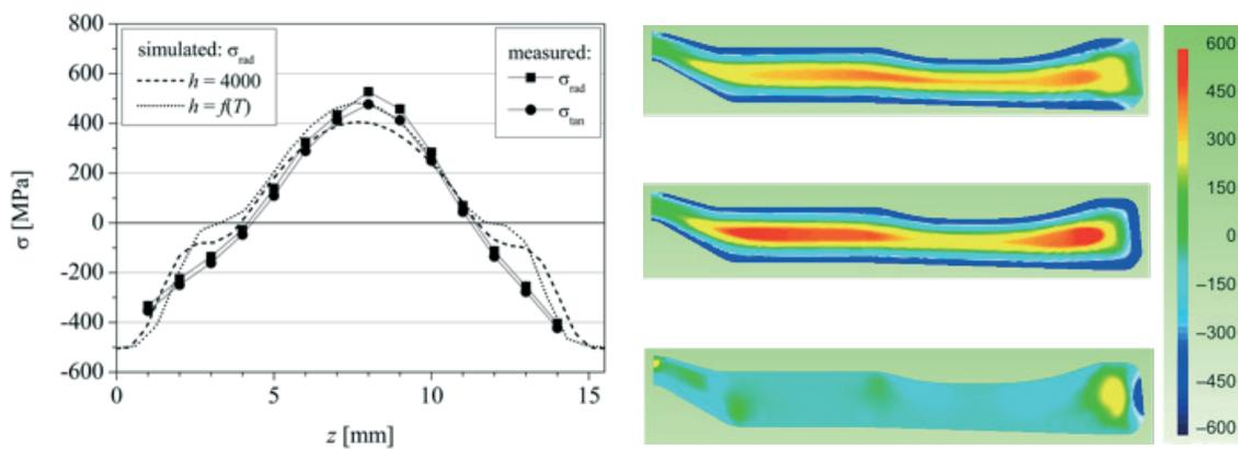
**Figure 2** Left: Residual stress distributions on the disc cross section after water quenching as predicted by the FE model. Right: Measured and calculated residual stress distribution through the thickness of a disc at the radius indicated by the dashed line in the left figure.
