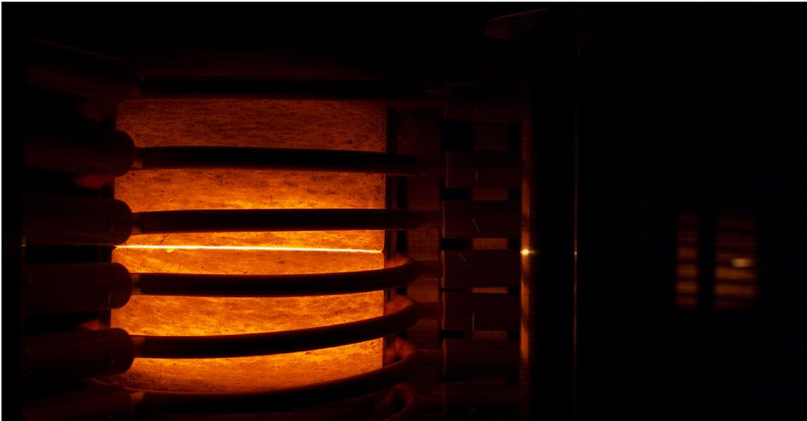
**Image** The high temperature graphene process uses induction heating to fabricate the material as precise as possible.
