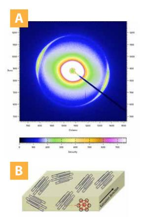
Figure 1 A) 2D SAXS pattern and B) proposed model, for the HCP scattering objects in extruded wheat gluten bioplastic films containing ammonium hydroxide and salicylic acid. Research with neutrons and photons has contributed to the development of a wide variety of products such as plastics, cosmetics, chemicals, building materials, life science and of course packaging materials. For example the paper wrapping of your hamburger or the milk carton in your fridge.
